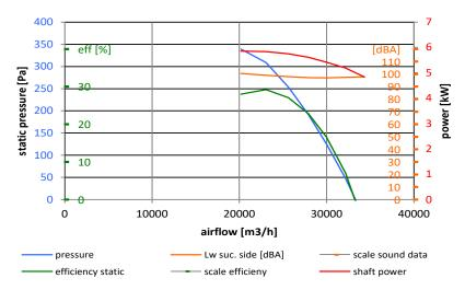
Measured in short casing with bellmouth without guard grille in installation type A according to ISO 5801.
