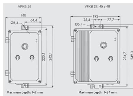
**The selection of the adjustable frequency drive has to be made with the maximum current absorbed of the fan or extractor.**
